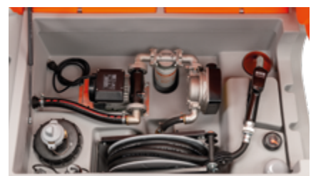
Outdoor Premium flow meter K33, filter with water separator, hose reel with 8 m hose DN 19, with hinged lid
