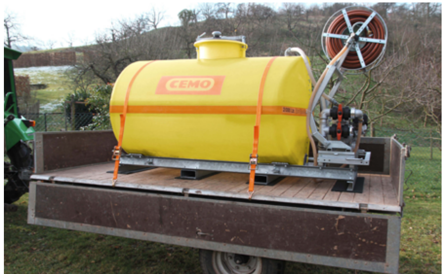
Securing loads with anti-slip mats and lashing straps (lashing down) using the example of a 2000-litre mobile irrigation system
