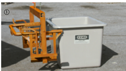
① Engaging the loading frame from the side after removal of the removable lid (shown with 700L grit bin)
