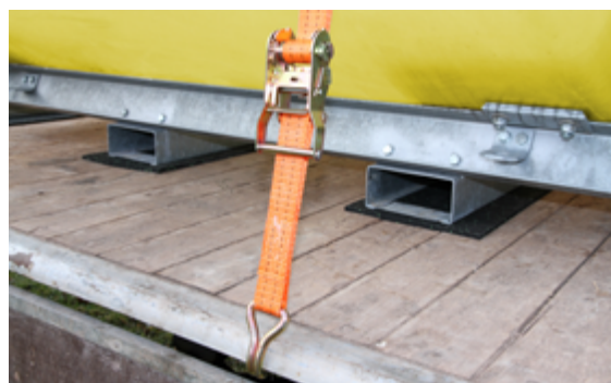
Securing loads with anti-slip mats and lashing straps (lashing down) using the example of a 2000-litre mobile irrigation system
