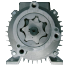
The pump principle: gear pump design
