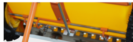
Rugged agitator shaft, axle divided in the middle
