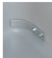
Platform fastening (reinforcement)
